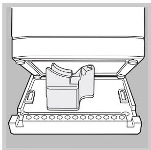
! This is a part of the polystyrene base and should have stayed intact when you removed the base.
