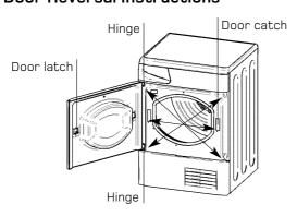
The door of your dryer is reversible and can easily be changed. Exchange diagonally hinge brackets and blanking screws. Exchange door latch and catch with their opposite blanking plates (see diagram above).
