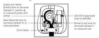
! If the plug being replaced is a non-rewirable type, then the cut-off plug must be disposed of safely. DO NOT leave it where it can be inserted into a socket and create a shock
