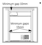
If you are going to install the appliance under a work counter, be sure to leave a 10mm space between the top and any other objects on or above the machine and a 15mm space between the sides and lateral furnishings or walls.
