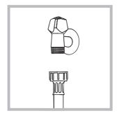
2. Connect the inlet hose by screwing it to a cold water tab using a 3/4 gas threaded connection (see figure).
