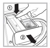
To remove the drawer, press lever (1) and pull the drawer outwards (2) (see figure). Wash it under running water; this procedure should be repeated frequently.
