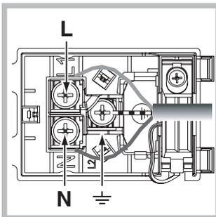
2. Install the power supply cable by loosening the cable clamp screw and the three wire contact screws L-N-. Connect the wires to the corresponding terminals: the Blue wire to the terminal marked (N), the Brown wire to the terminal marked (L) and the Yellow/Green wire to the terminal
