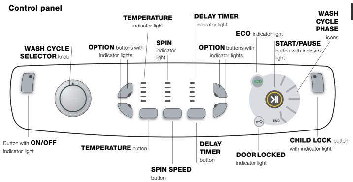
Button with () **ON/OFF** indicator light: press this briefly to switch the machine on or off. The green indicator light indicates that the machine is switched on. To switch off the washing machine during the wash cycle, press and hold the button for approximately 3 seconds; if the button is pressed briefly or accidentally the machine will not switch off. If the machine is switched off during a wash cycle, this wash cycle will be cancelled.
