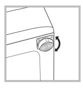
2. If the floor is uneven, the front feet of the machine may be adjusted until it reaches a horizontal position (the angle of inclination must not exceed 2 degrees).
